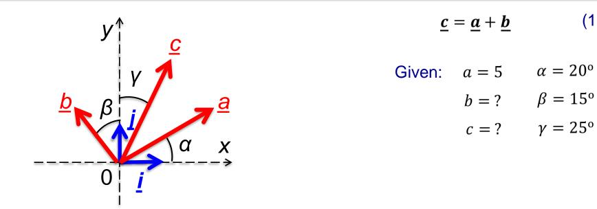
$\rightarrow^+ \Sigma X: c_x = a_x + b_x \rightarrow c \sin \gamma = a \cos \alpha - b \sin \beta$  $\uparrow^+ \Sigma Y: \ c_v = a_v + b_v \rightarrow c \cos \gamma = a \sin \alpha + b \cos \beta$  $\begin{bmatrix} 0.2588 & 0.4226 \\ -0.9659 & 0.9063 \end{bmatrix} \begin{pmatrix} b \\ c \end{pmatrix} = \begin{pmatrix} 4.698 \\ 1.710 \end{pmatrix}$
